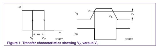
Built in DC hysteresis in logic devices is useful in systems where inputs have some noise due to electromagnetic induction, or cross talk etc. Each input has immunity against noise depending on the amount of hysteresis voltage present.
